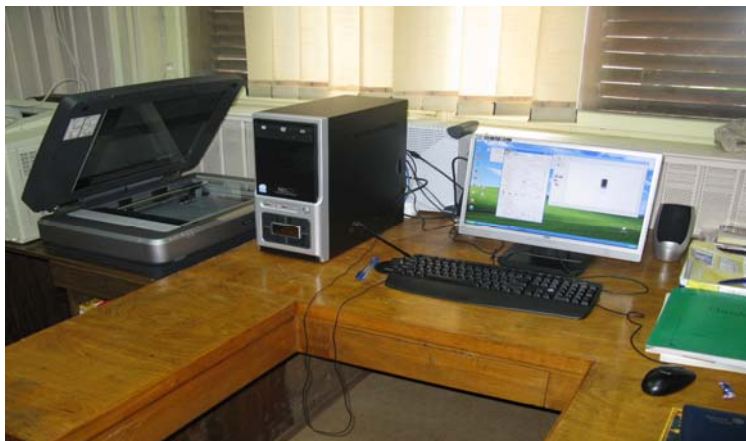
Figure 7. The Rozhen Observatory EPSON Expression 10000XL (A3) professional flatbed scanner.
