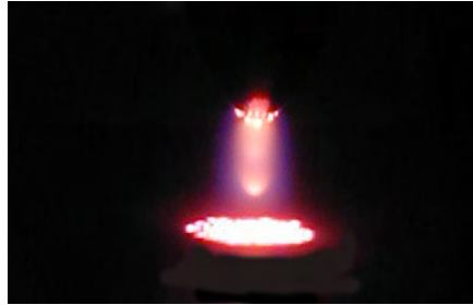
Fig. 1. Photo of the APGD in helium.
